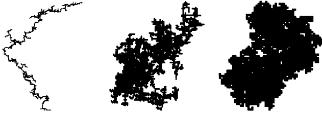
FIG. 1. Two-dimensional projections of typical aggregates of 8192 particles built with the variable- D cluster-cluster hierarchical procedure with D = 1.5, 2, 2.5 . The scale has been chosen such that the vertical size is the same in all pictures.
